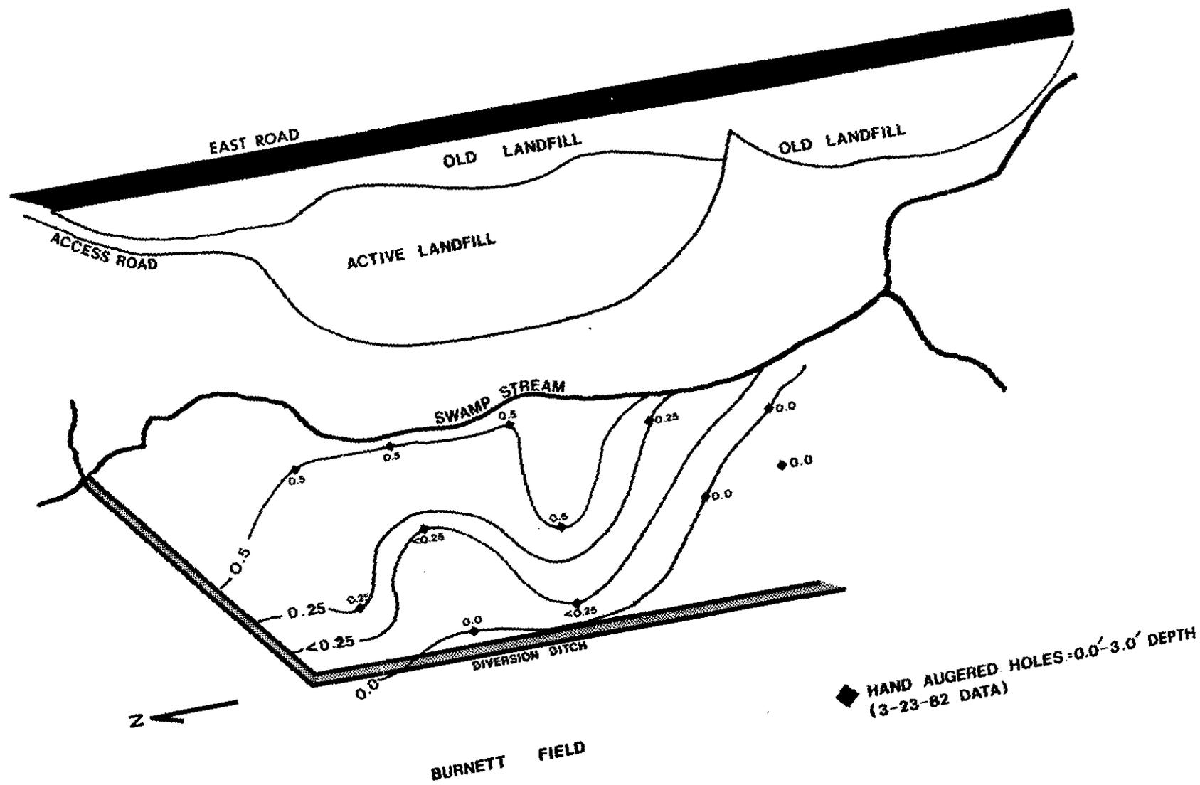
Figure 5. Adams Landfill: Plan View; Salinity Contours
