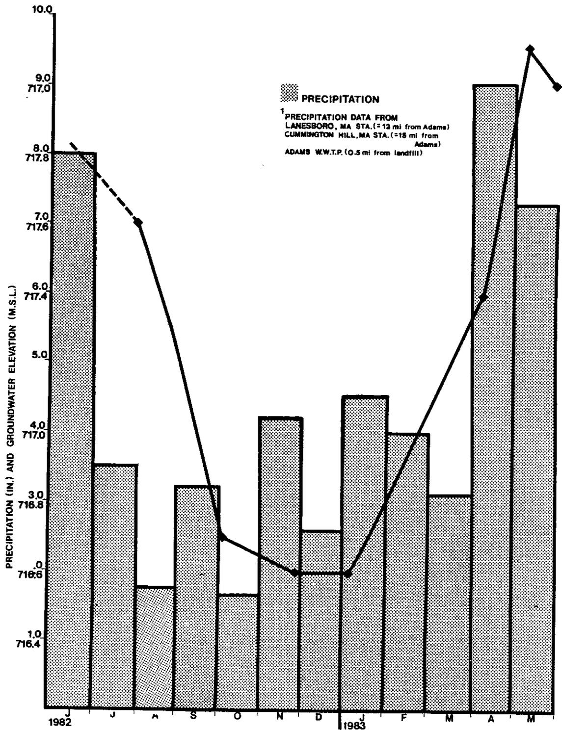
Figure 28. Precipitation (1982-83) vs Groundwater Elevation (Well #3)
