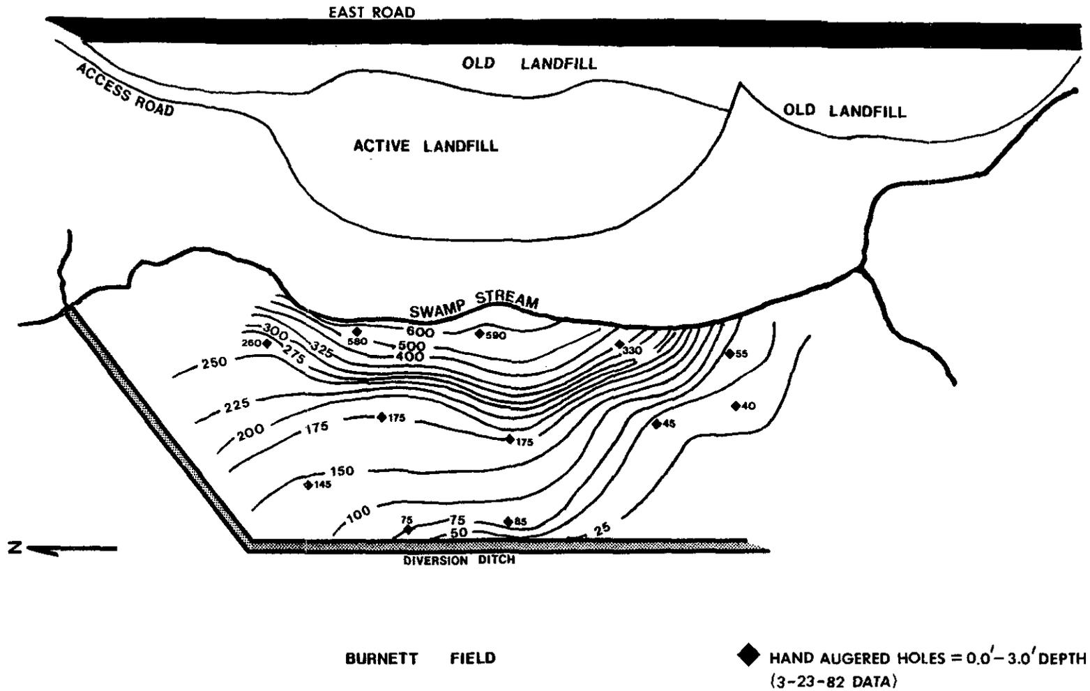
Figure 3. Adams Landfill: Plan View; Specific Conductance Contours
