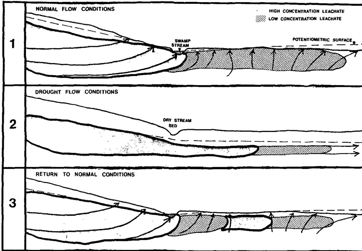
Figure 31. Possible Explanation for the Presence of an Isolated Zone of High Concentration
