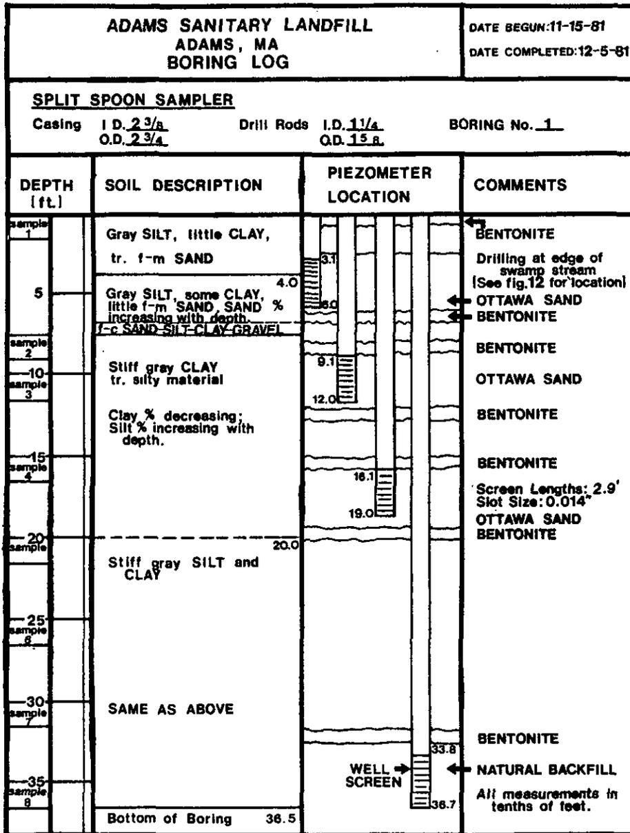
Figure 8. Adams Sanitary Landfill: Boring Log; Well #1
