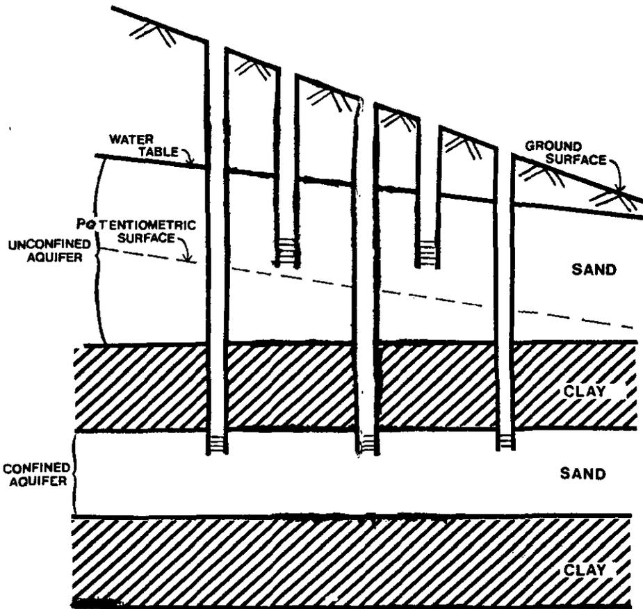
Figure 29. Confined and Unconfined Aquifers
