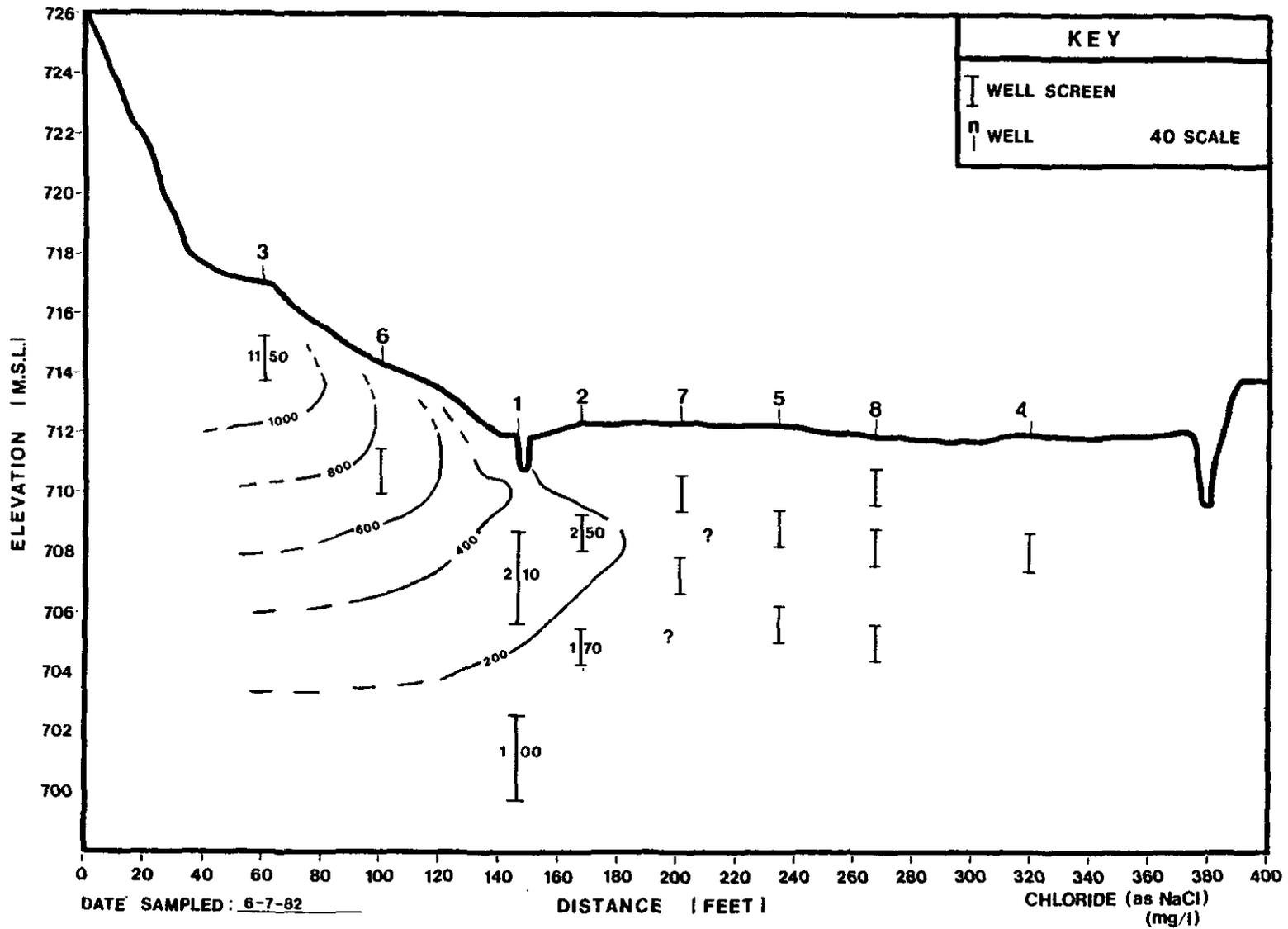
Figure 10. Concentration Data and Plume Location: Wells 1, 2 and 3
