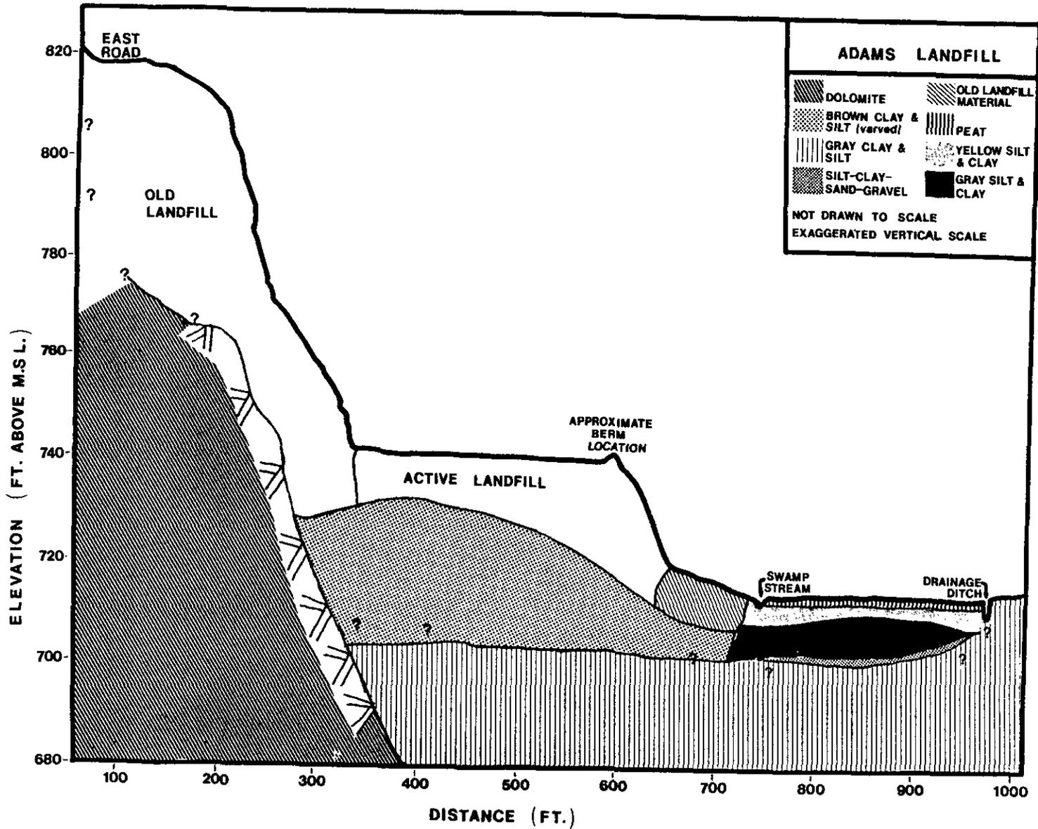
Figure 2. Adams Landfill: Section View
