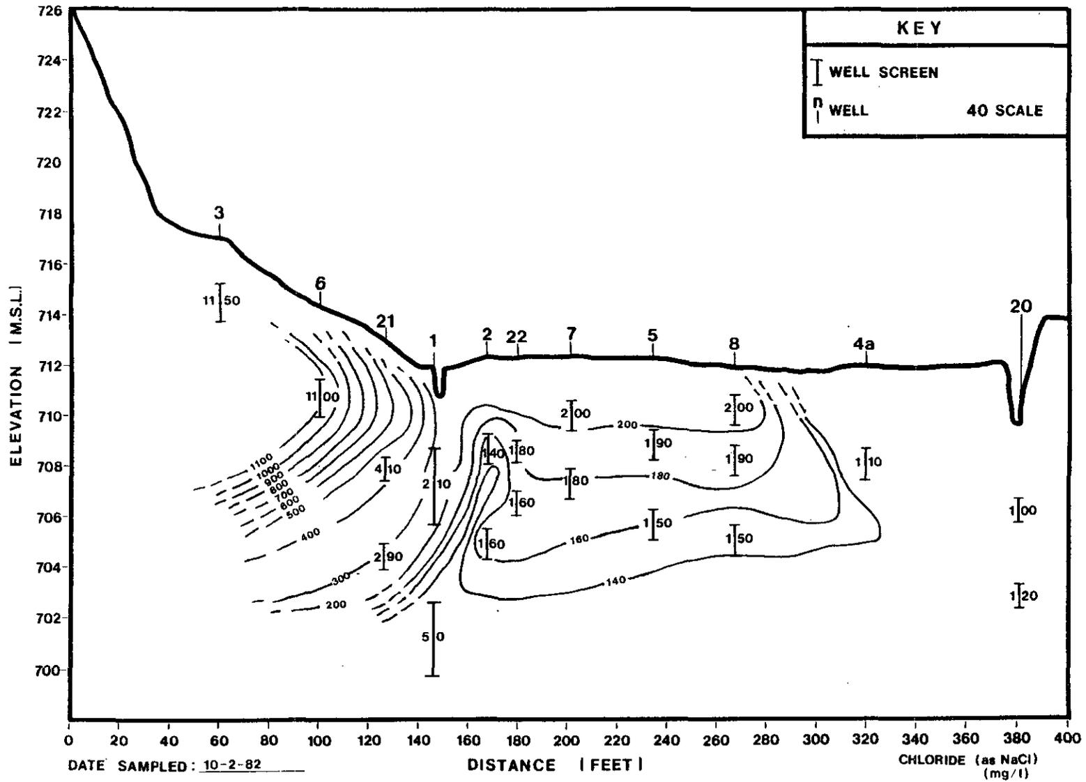
Figure 30. Profile of Chloride Concentrations along Main Well Line
