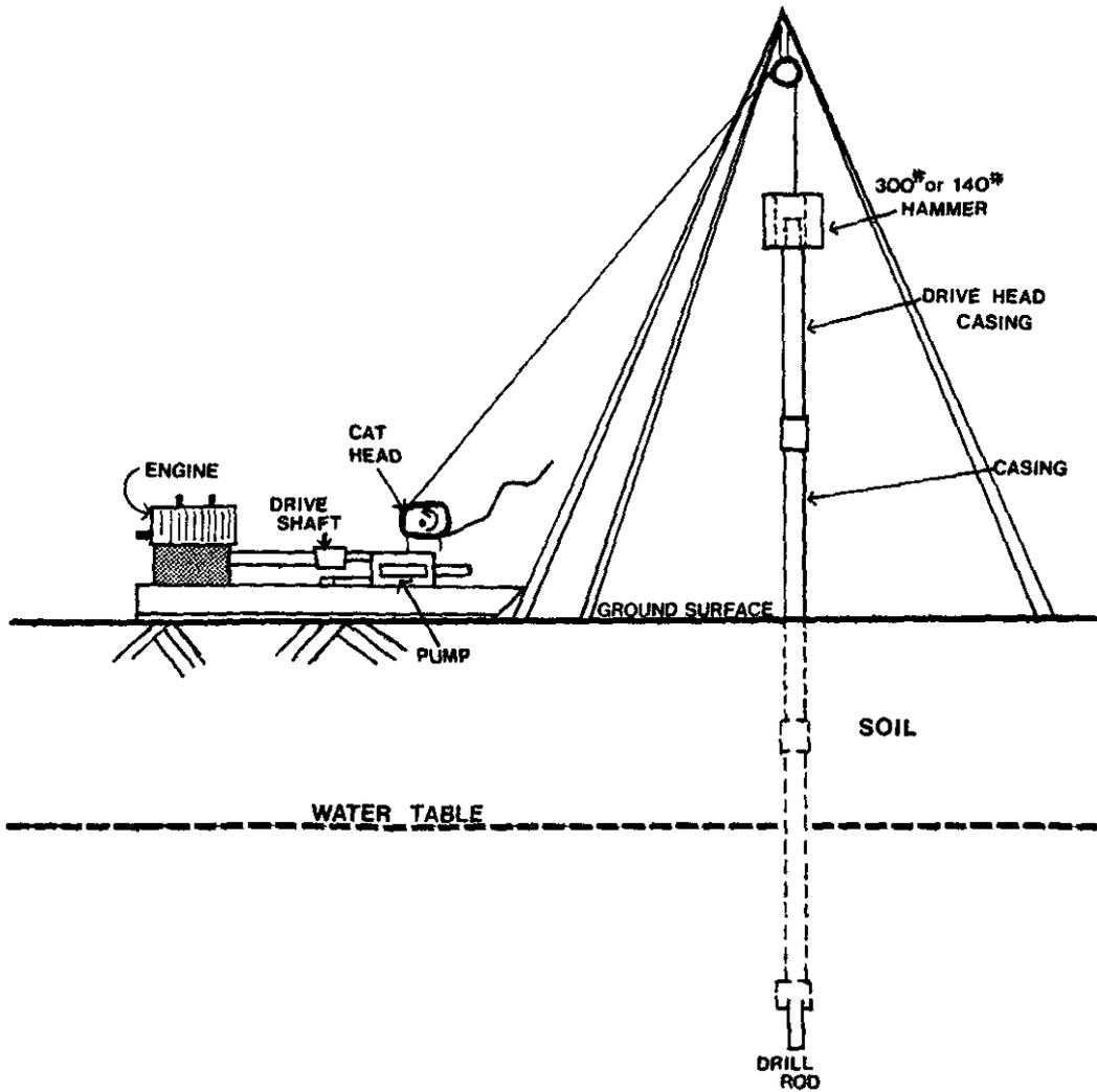
Figure 7. Wash Boring Drilling Rig
