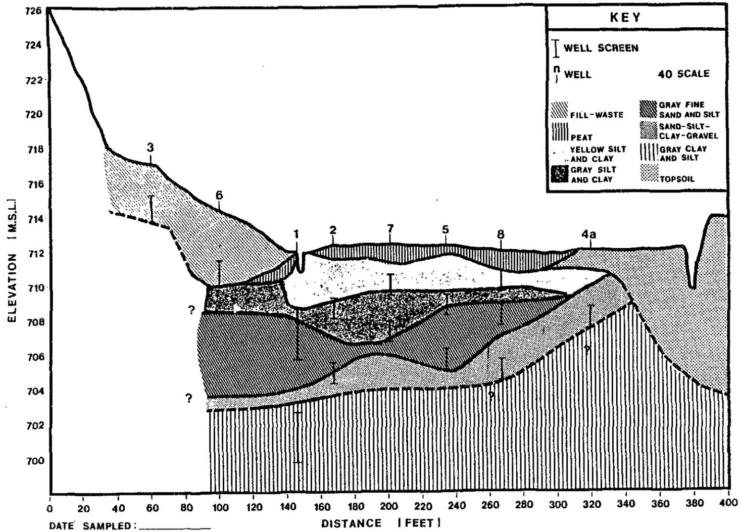
Figure 9. Well Location: Section View along the Central Line of Wells
