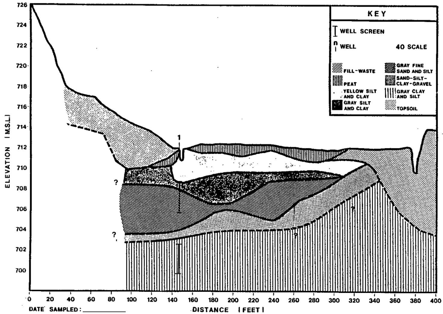
Figure 6. Complete Section View of Main Well Line (Well screens from 16-19 and 33.7-36.7 feet not shown. Gray silt and clay continued until 36.7 feet.)
