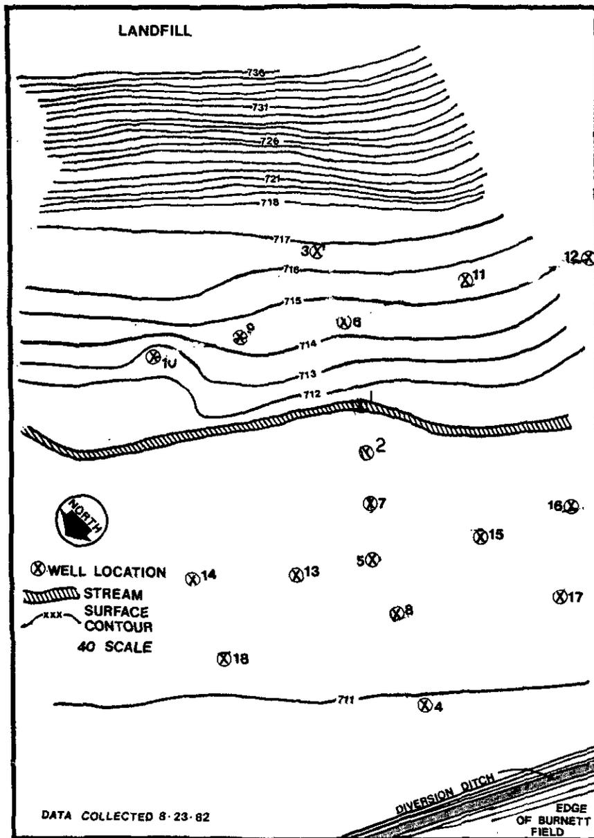
Figure 12. Adams Landfill: Surface Contours and Well Locations
