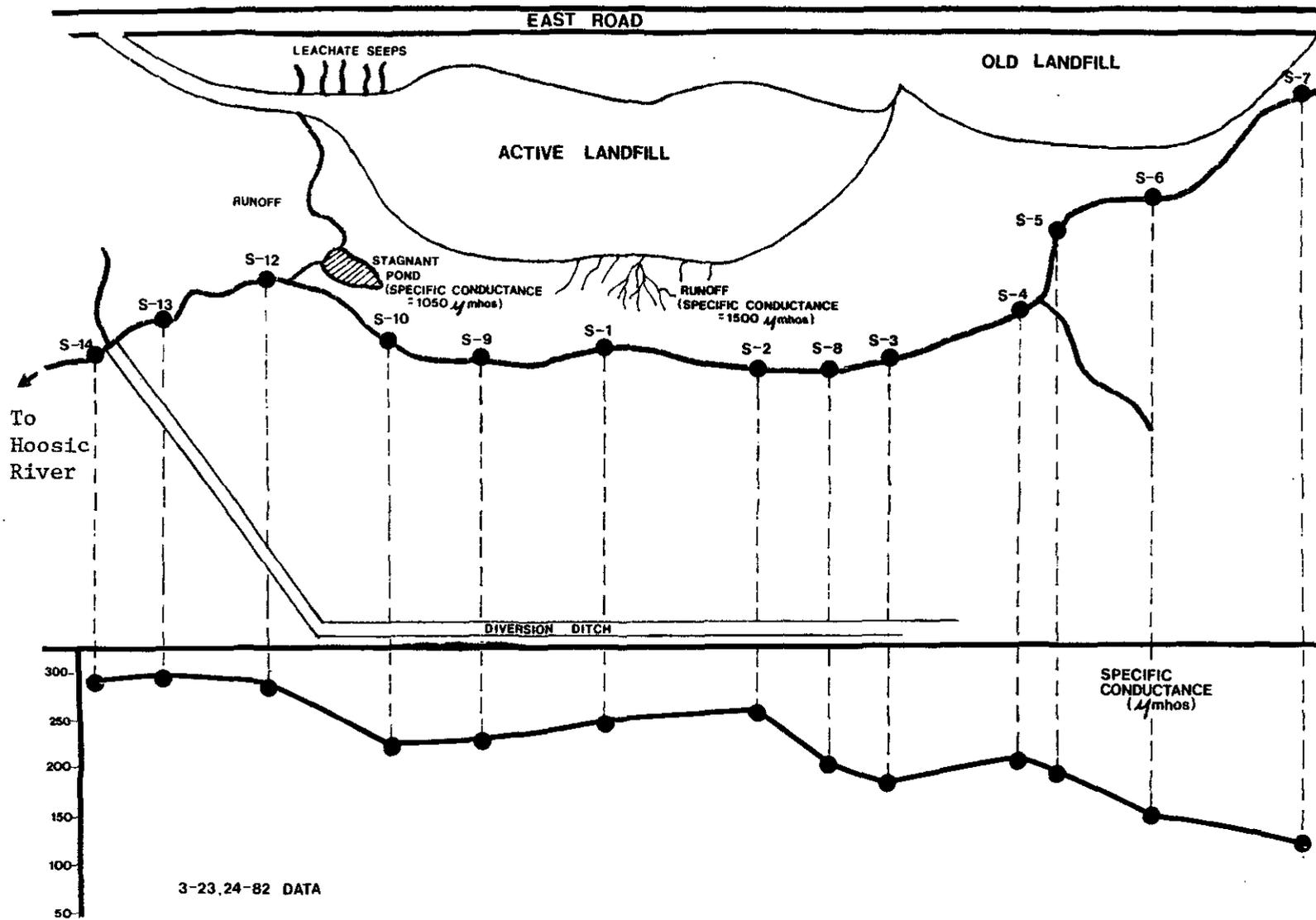
Figure 34. Adams Landfill: Specific Conductance in Swamp Stream
