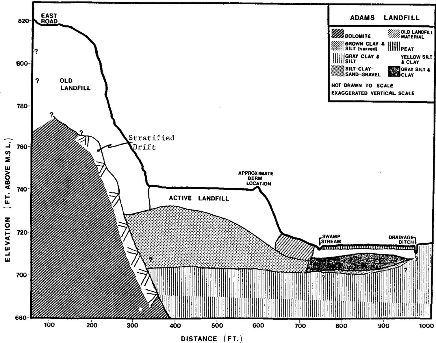
Figure 23. Adams Landfill; Section View
